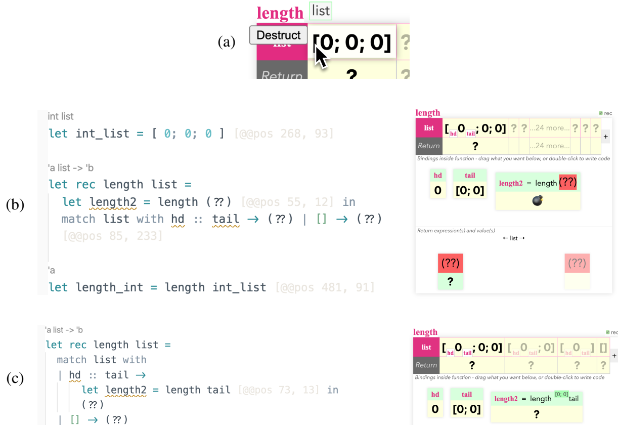
Figure 4.8: (a) A “Destruct” button appears when the cursor hovers over an input value that is an ADT. (b) Code and length function TV after destructing on the [0; 0; 0] input value. (c) After dragging the tail value [0; 0] to the red hole argument (??) for the recursive length call.
