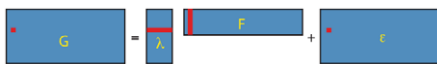
Figure 1. Low-dimensional matrix factorization via factor analysis. Each matrix in Equation 1 is illustrated by a blue rectangle and labeled. As in Equation 2, a single element of genotype matrix G , G_{i,j} is shown in red, and is computed from the product of the appropriate factor loading and factor vectors plus the corresponding random error term (all highlighted in red). doi:10.1371/journal.pgen.1001117.g001
