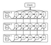
Model parallel training, where different portions of the model computation are done on different computational devices simultaneously for the same batch of examples. For example: A recurrent, deep LSTM model used for sequence to sequence learning, parallelized across three different devices.
