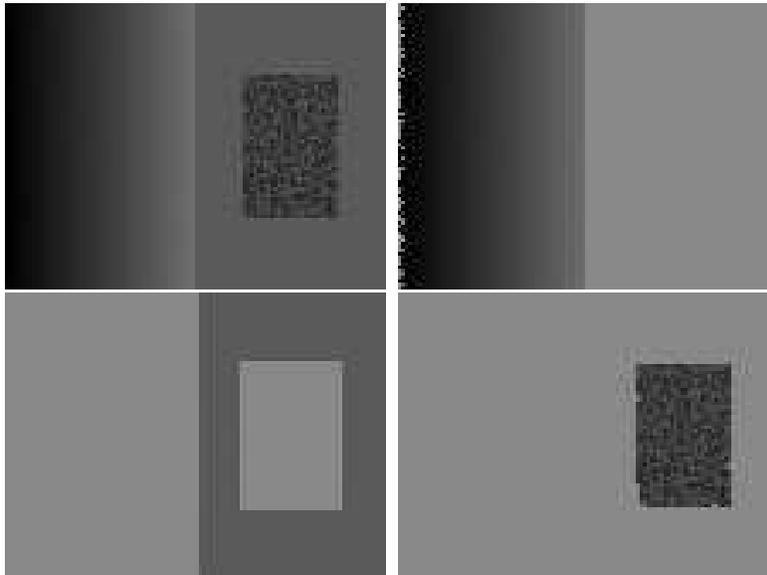
Figure 1: A synthetic image with three perceptually distinct regions, and the three largest regions found by our segmentation method (image  $320 \times 240$  pixels; algorithm parameters  $\sigma = 0.8$ ,  $k = 300$ , see Section 5 for an explanation of the parameters).
