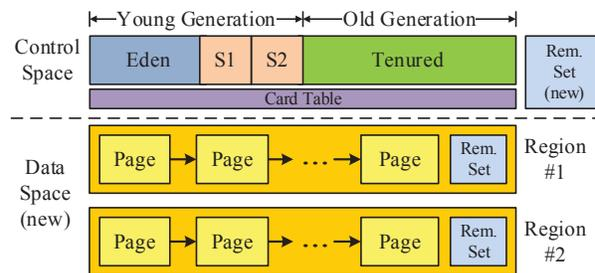
Figure 6: The heap layout in Yak.
