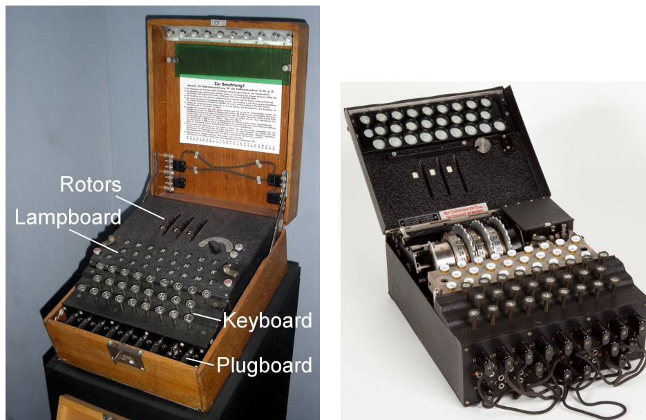
Figure 2.1: Two images of Enigma. Credit: Left image by Karsten Sperling (public domain, downloaded at https://commons.wikimedia.org/wiki/File:EnigmaMachineLabeled.jpg , Right image by Alessandro Nassiri ( https://creativecommons.org/licenses/by-sa/4.0/deed.en , no changes.)
