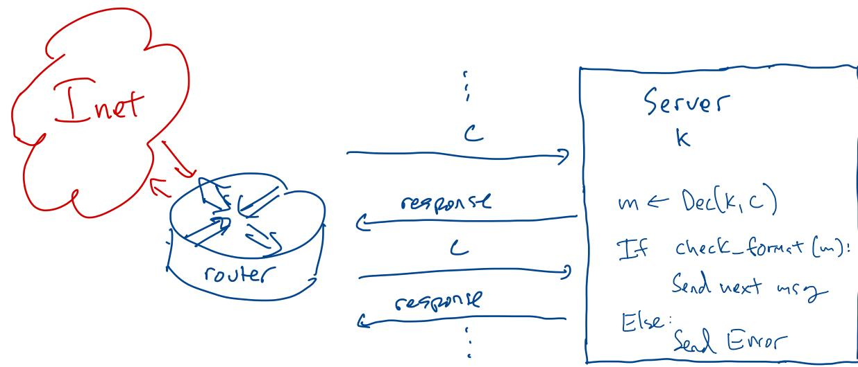
A typical attack setting: Server connected to the Internet
