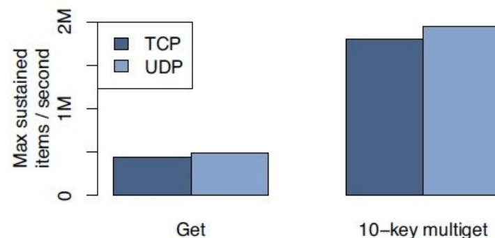
Figure 8: Get hit performance comparison for single gets and 10-key multigets over TCP and UDP
