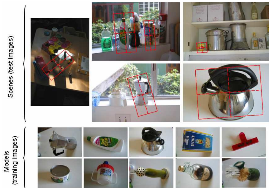
Fig. 5. Samples from our training and test sets. The red boxes show locations where models were identified
