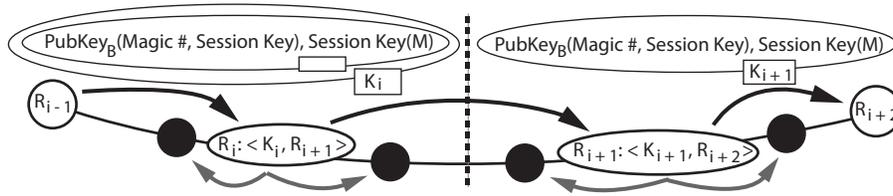
Fig. 2. Message decryption in Bluemoon. Each relay group root removes a layer of encryption using its symmetric key  $K_i$ , and forwards the message to the next relay group  $R_{i+1}$  and to the other members of its group.
