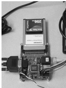
Figure 2: Our target board. The Stargate is a small sensor network gateway running Linux, and is almost same as an HP iPAQ.
