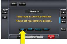
6. (optional: if you want audio) If you wish to hear audio from your laptop, you can either configure your laptop to send audio to the HDMI port (which will appear as "Extron Scaler") or use a VGA connection and the 3.5mm jack for audio. In addition to the controls on your laptop, the audio volume can be controlled or muted using the controls at the right side of the touch screen.
